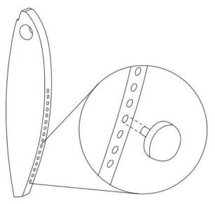
The 'Disc Support Nodule' is a spherical rubbery support. It is intended to support a slipped disc (Herniated disc) and can be inserted into any of the numbered holes on the 'spine profile' according the user's preferred height position. It protrudes from the 'spine profile' curve and provides support to the individual slipped disc.
